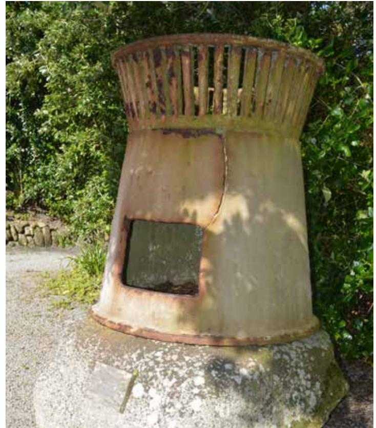
ABOVE LEFT: The St. Agnes lighthouse (1680) on the Isles of Scilly which was lit by coal burned in the cast iron chaffer (grate) ABOVE RIGHT. The unique item can be seen in the gardens of Tresco Abbey.
